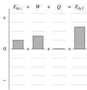
**Solve:** This is an adiabatic process of gas compression so no heat energy is transferred between the gas and the environment. That is, Q = 0 J. According to the first law of thermodynamics, the work done on a gas in an adiabatic process goes entirely to changing the thermal energy of the gas. The work W is positive because the gas is compressed.
